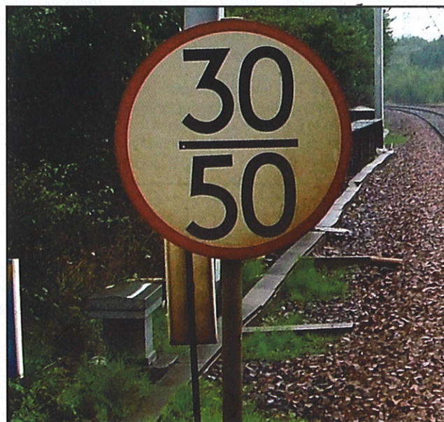
Example of a differential speed sign. Photo © Mott MacDonald 2004.
