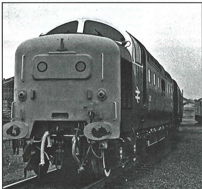
In 1961 the 3300hp Deltic fleet began to be introduced, becoming the backbone of the East Coast Main Line fleet until the arrival of the HST sets in 1977.
