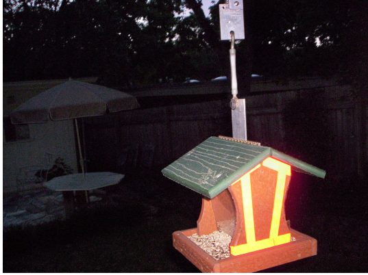
Fig. 2 Flash picture of bird feeder. Note that the retroreflective tape is very bright, even though the angle with the normal is close to 30 degrees ( \text{ATAN}(8 \text{ in.}/4 \text{ in.}) = 27^\circ ).
