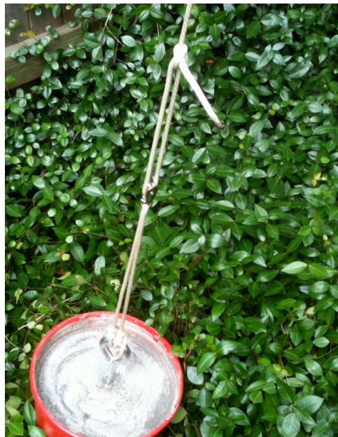
Fig. 16 35 lb. Counterweight, pulley # 3 and taut line hitch
