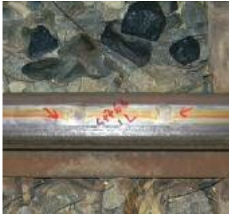
Figure 6: below: on viaduct R=3000 curve, above: a squat with a wave at tangent track, Photos Izmir Metro archive 2010.
