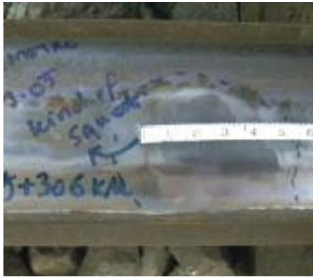
Figure 6: below: on viaduct R=3000 curve, above: a squat with a wave at tangent track, Photos Izmir Metro archive 2010.
