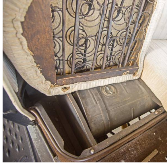
Lizzie's passenger seat gas tank.
